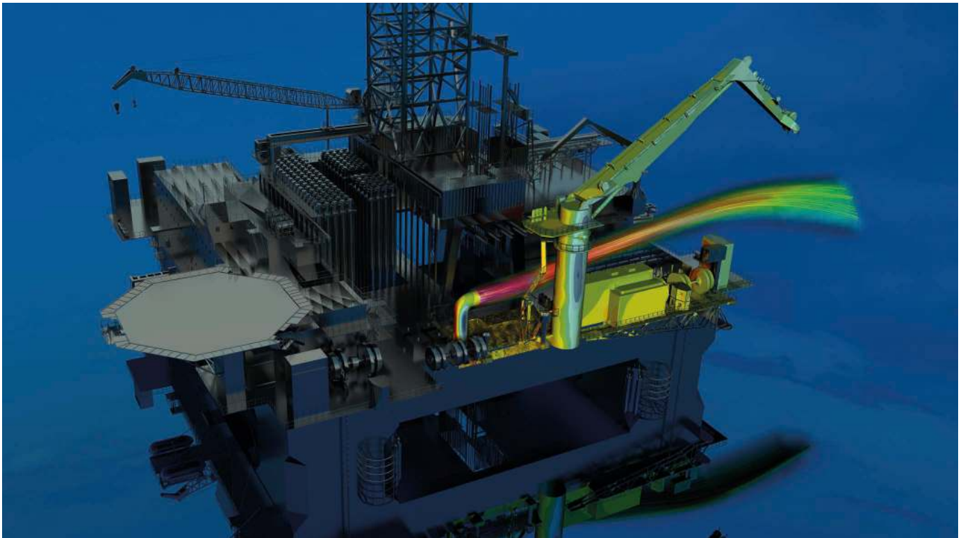
Gas dispersion safety study of an offshore floating platform.
