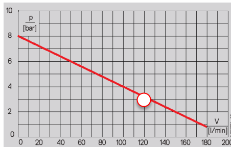
Pump performance curve
